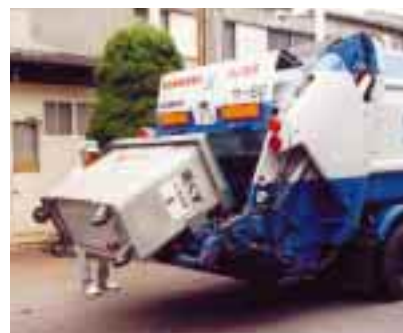
Waste collection truck with automatic scale
