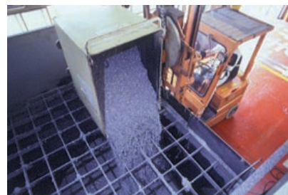
In-house aluminum file dust recycling Above: Recovered file dust is placed in this hopper. Right: File dust is melted down in this smelter.
