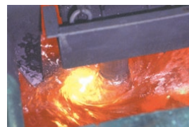
In-house aluminum file dust recycling Above: Recovered file dust is placed in this hopper. Right: File dust is melted down in this smelter.
