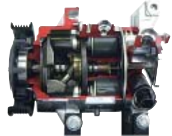
Car air conditioning compressor incorporating adjustment control unit
