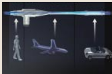
This ejector, in which refrigerant can travel at dramatically different speeds, was made possible through proprietary numerical analysis and manufacturing technology.
