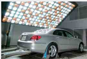
Thermal testing simulating conditions at the equator
